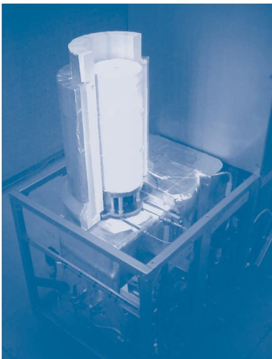
*A stack of fuel cells incorporated in CFCLs prototype CHP unit (combined heat and power).*
