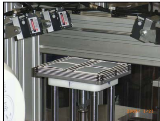
Figure 7 - Robotic Assembly of Fuel Cells
