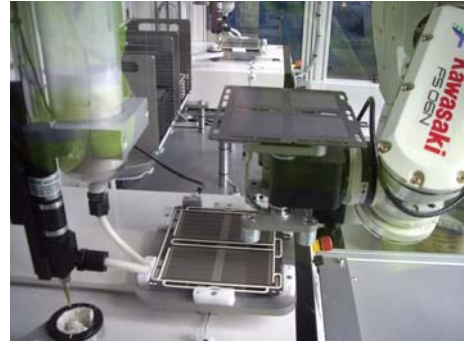
Figure 5 - Automated Seal Dispensing
