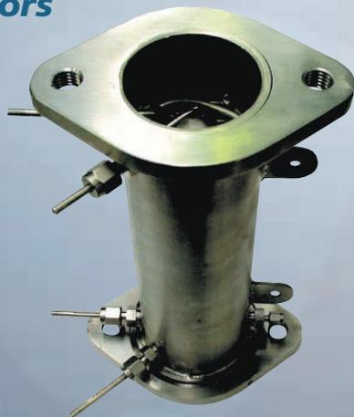
system. The design allows for instantaneous generation of steam to meet the demands of the fuel cell process. The steam generator is able to operate over a wide range of flows and temperatures on both gas and liquid sides. A 420 watt steam generator is illustrated.
