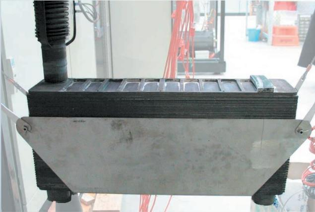
5.5 kW Air-to-Air Heat Exchanger
